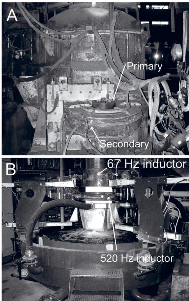
Fig. 1. **A:** induction furnace operating at 50 Hz. In the foreground, the step-down transformer is visible, with the secondary winding clad in heat-resistant material. **B:** The induction hardening machine with two single-winding inductors.
