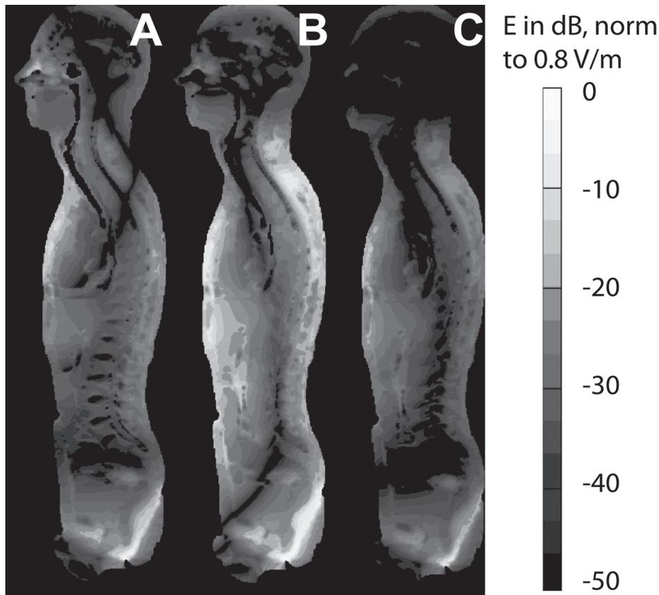
Fig. 2. Induced electric field in dB normalized to 0.8 V/m for the exposure at: (A) 50 cm from the induction hardening machine at 67 Hz, (B) at 50 cm from the induction hardening machine at 520 Hz, (C) at 30 cm from the induction furnace at 50 Hz.
