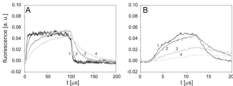
FIGURE 3 Time response of the imaging system on a step change of the light from a green LED. Durations of the LED signal were set to (A) 100  $\mu$ s, and (B) 10  $\mu$ s. Bandwidths of the amplifier: (1) 117 kHz, (2) 39 kHz, (3) 7.7 kHz, and (4) 3.5 kHz.
