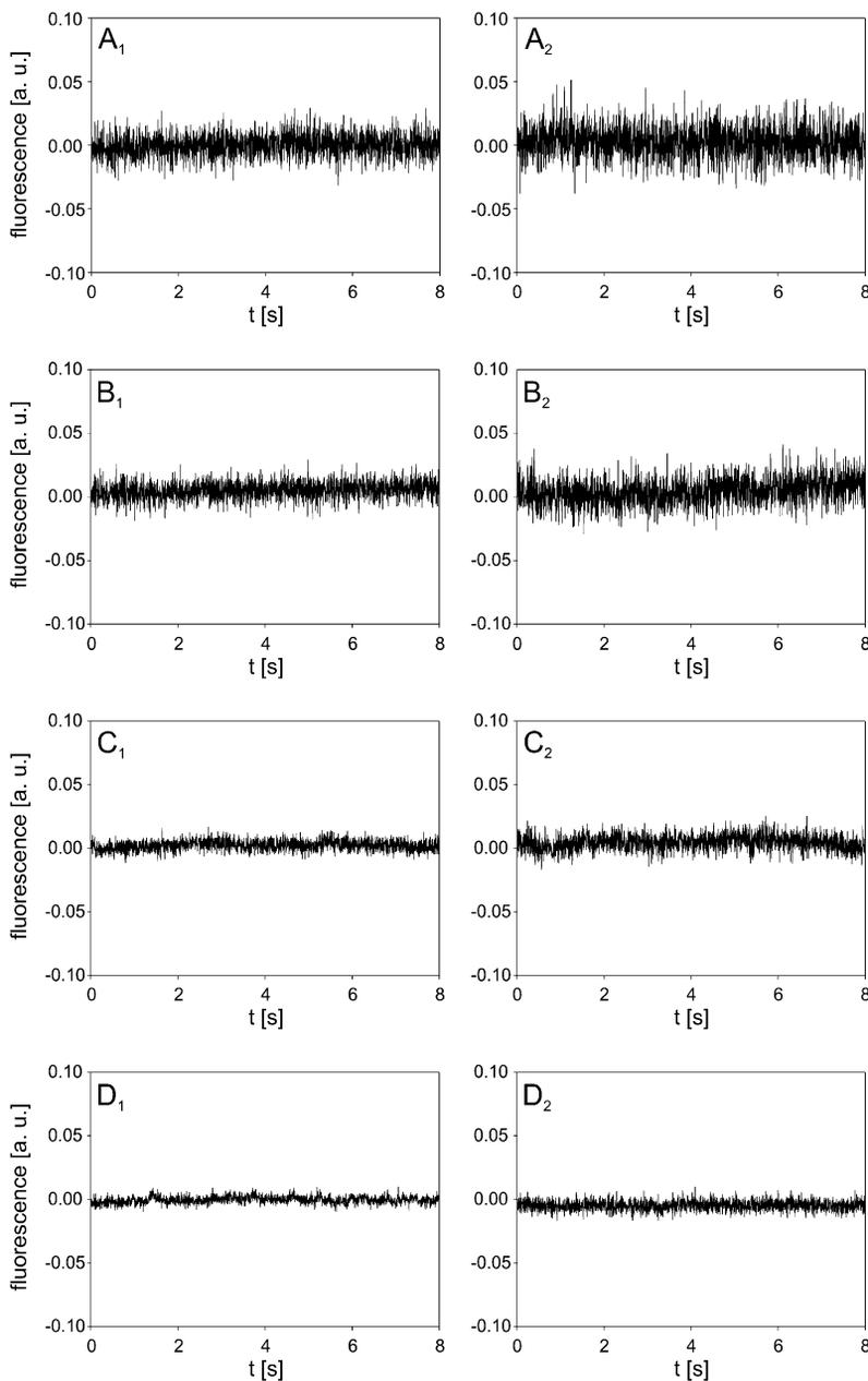
FIGURE 2 Noise analysis. (Left column) Noise in solution of 100  $\mu$ M PI. (Right column) Noise in suspension of cells and 100  $\mu$ M PI. The measurements were performed at (A) 117 kHz, (B) 39 kHz, (C) 7.7 kHz, and (D) 3.5 kHz bandwidth of the amplifier. The background fluorescence of the solution was subtracted by the differential acquisition of the signal.
