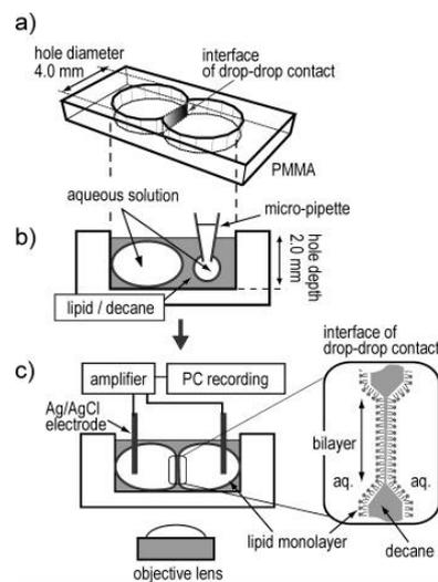
**Figure 7: a) Overview of the double well chip, consisting of two wells connected. b) Procedure of the bilayer formation. Two droplets are injected in each well filled with lipid solution, forming a water/lipid solution/water interface at the section. c) Schematic diagram of the experimental setup. Electrodes are inserted in each droplet, and membrane current is measured using a patch clamp amplifier. (Funakoshi et al. 2006).**
