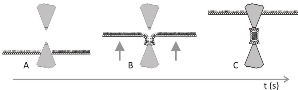
**Figure 5: Folding method. A) The lipid monolayers on the surface of liquid solution below the aperture. B) The surfaces of liquid solutions are crossing the aperture and forming planar lipid bilayer. C) Planar lipid bilayer is formed.**
