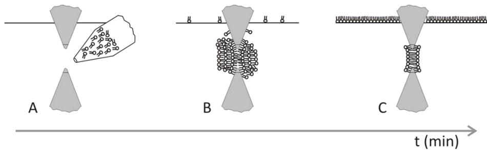
**Figure 4: Painting method. A) Aperture and tip filled with lipid solution. B) Cluster of lipids on aperture. C) Planar lipid bilayer is formed.**
