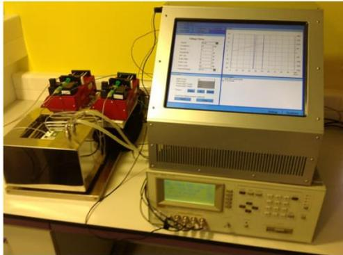
**Fig. 1** The photography of the system for measuring the properties of planar lipid bilayers. On the left are two pumps for filling reservoirs and the bath with temperature regulation. The measurement chamber with four electrodes is inserted into the bath. The cables from the electrodes lead to the control unit, which is on the right. Below the control unit is the LCR meter
