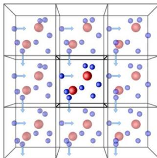
**Figure 9: Scheme of periodic boundary conditions.**
