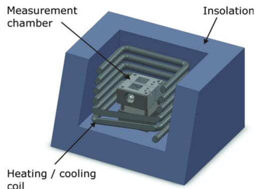
**Fig. 5** The temperature-regulated bath with the measurement chamber. The bath is constructed of stainless steel and insulation. The heating coil and the measurement chamber are inserted into the bath
