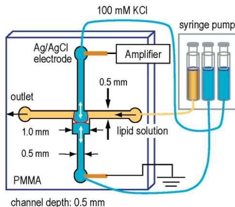
**Figure 8: Schematic of the cross-channel chip. Two aqueous solutions with lipid solution in between make contact at the cross section to form a lipid bilayer (Funakoshi et al. 2006).**
