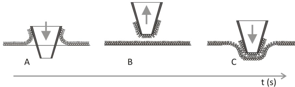
**Figure 6: Tip-dip method. A) The tip is in the liquid solution. B) The tip is pulled out of the liquid solution. C) The tip is pushed back in the solution.**
