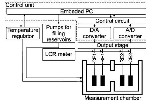
**Fig. 2** The system for measuring the properties of planar lipid bilayer consists of the control unit, the LCR meter, the output stage, the pumps for filling reservoirs, the measurement chamber with four electrodes and the bath with temperature regulation. The control unit consists of the embedded PC, the control circuit, the digital to analog converter and the analog to digital converter
