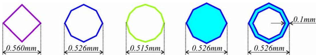
Figure 4.3: Cross section of 4, 8 and 12 faceted, solid and tube electrodes.
